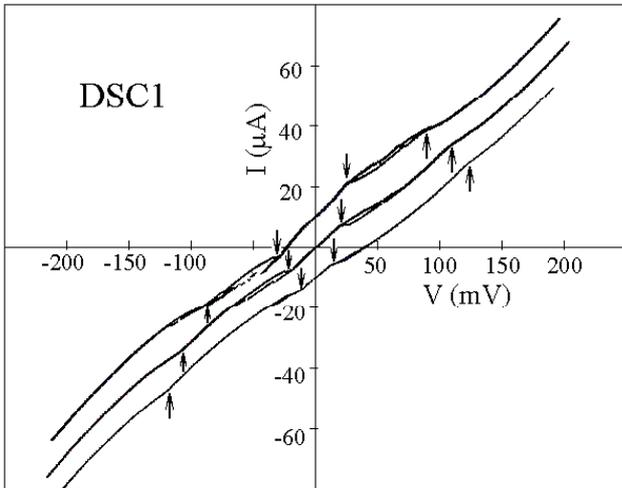
**Figure 5.** Variation of  $I$ - $V$  characteristics of the sample DSC1, for external magnetic fields of  $H = 3.0, 4.0$  and  $5.0$  T, which clearly show the low- and high-voltage cusps. For clarity, the  $3.0$  T curve ( $5.0$  T curve) was shifted upward (downward) by  $10 \mu\text{A}$ .
