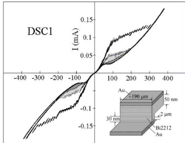
**Figure 4.** Variation of  $I$ - $V$  characteristics of the sample DSC1, for external magnetic fields of  $H = 0.5, 1.0$  and  $2.0$  T, fabricated by removing the main part of the pedestal stack.
