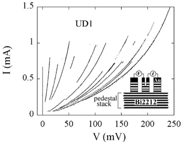
**Figure 1.** Zero-field  $I$ - $V$  curves taken at  $T = 4.2$  K of the mesa UD1 which contains 12 intrinsic junctions. Inset: a four-terminal measurement configuration for the central mesa of the lateral dimensions of  $10 \times 45 \mu\text{m}^2$ .
