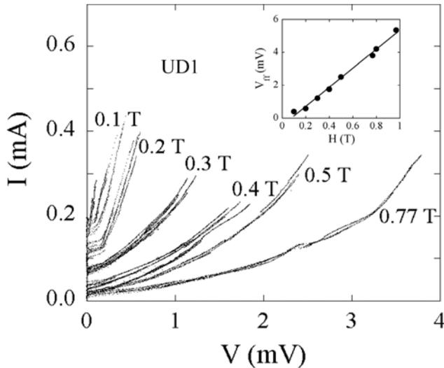
**Figure 2.** The evolution of the supercurrent branch of the mesa UD1 in low dc magnetic fields between 0.1 T and 0.77 T. The inset shows a linear magnetic-field dependence of the flux-flow voltage  $V_{ff}$ .
