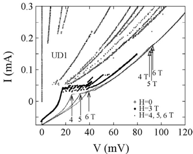
**Figure 3.**  $I$ - $V$  characteristics of the mesa UD1 in dc magnetic fields of  $H = 0, 3, 4, 5$  and  $6$  T. The curve for  $3$  T (the ones for  $4, 5$  and  $6$  T) is shifted downward by  $0.065$  mA (by  $0.075$  mA) for the clarity of illustration.
