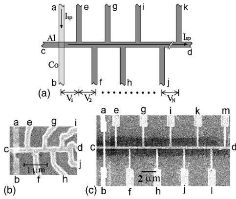
FIG. 1. (a) Schematic geometry of the samples. SEM micrographs of (b) sample A and (c) sample B.
