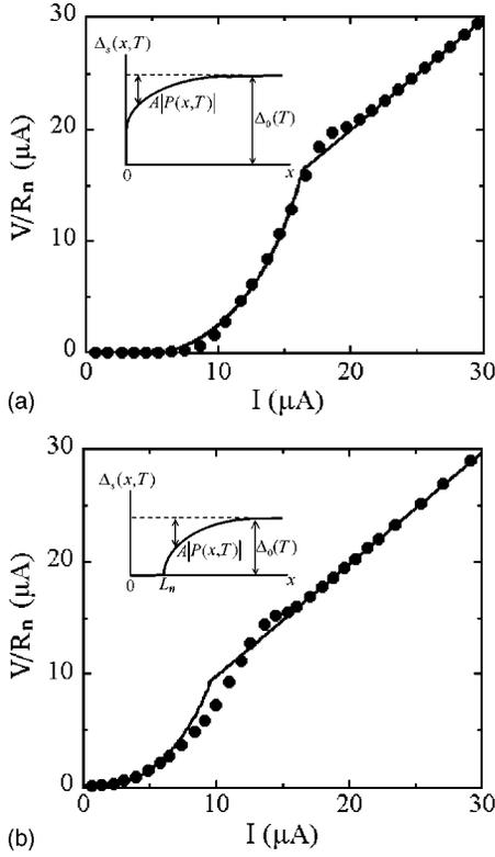
FIG. 7.  $I$ - $V$  characteristics (open circles) of segment 1 for temperatures (a) far below  $T_c$  ( $T=0.1$  K) (b) and near  $T_c$  ( $T=1.3$  K) in sample A, with the best-fit curves (solid curve) using Eqs. (2) and (3).
