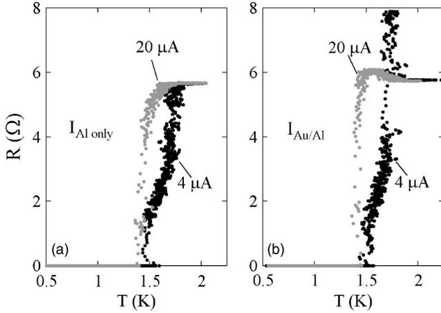
FIG. 6. The resistive transition of segment 1 of the Al wire in a Au/Al hybrid sample for the bias current applied (a) only through the Al wire and (b) through the Au/Al interface from the Au wire, each for the low and high bias levels.
