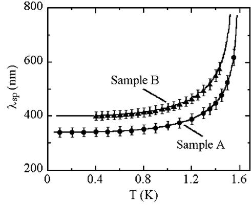
FIG. 8. The temperature dependence of  $\lambda_{sp}$  for samples A (circles) and B (triangles), extracted from the best-fit curves in  $I$ - $V$  characteristics based on Eqs. (2) and (3). The solid curves are the best fits to the relation  $\lambda_{sp}=\sqrt{D\tau_{sp}}$ , together with Eq. (4).
