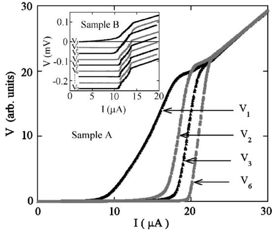
FIG. 4.  $I$ - $V$  characteristics of sample A taken at 0.10 K, along segments 1, 2, 3, and 6 of the Al wire for the spin-injection bias configuration. Inset: The spatial dependence of the  $I$ - $V$  characteristics taken from segments 1, 2, ..., 9 of the Al wire of sample B at 0.43 K. For clarity each curve is offset downward from the nearest neighbor by 0.03 mV.
