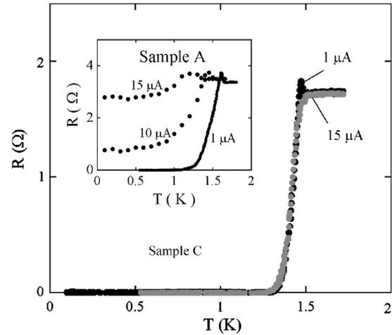
FIG. 3. The resistive transition of segment 1 of the Al wire in sample C, consisting of a Au/Al junction, for the bias currents of  $1$  and  $15 \mu\text{A}$ . Inset: The resistive transition of segment 1 of the Al wire of sample A for increasing spin-polarized bias current from  $1$  to  $15 \mu\text{A}$ .
