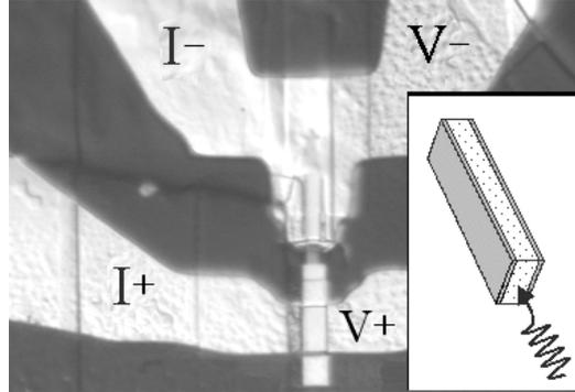
FIG. 1: Optical micrograph of a stack fabricated by the double-side-cleaving technique. The inset shows the direction of microwaves irradiation to the sample.
