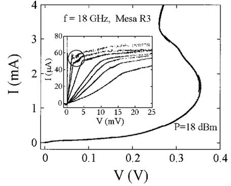
FIG. 4.  $I$ - $V$  characteristics with irradiation of a microwave of frequency  $f=18$  GHz and power  $P=18$  dBm. Inset: detailed view of the low-bias flux-flow branches with microwave power of  $P=5, 8, 10, 12, 13, 15, 16,$  and  $18$  dBm, from left to right.
