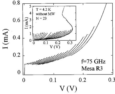
FIG. 1.  $I$ - $V$  curves of mesa R3 at  $T=4.2$  K with irradiation of a microwave of  $f=75$  GHz and power  $P=17.7$  dBm. Inset:  $I$ - $V$  curves without irradiation of a microwave. The total number of IJJ's in the mesa is  $N=23$ .
