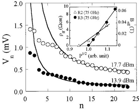
FIG. 3. The cutoff voltage  $V_n$  as a function of the mode index  $n$  for  $P=13.9$  (filled circle) and  $17.7$  dBm (open circle). The filled lines are calculated results using Eq. (1) with the Swihart velocity as the fitting parameter. Inset: microwave power dependence of the flux-flow resistivity  $\rho_{ff}$  and  $B_{eff}$ . The lines are guides to the eyes.
