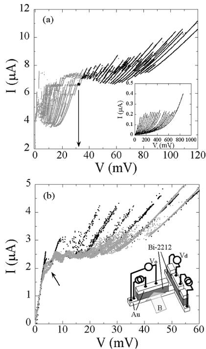
**FIGURE 1.** (a) Josephson vortex-flow branches (grey curves) and the quasiparticle branches (black curves) of the oscillator stack in  $B=2.5$  T. The inset of (a): the current-voltage curves of the oscillator stack in zero field. (b) The quasiparticle branches of detector stack in  $B=2.5$  T, without a bias (black curves) and with a bias of 32 mV (grey curves) to the oscillator stack. The inset of (b): the sample configuration.
