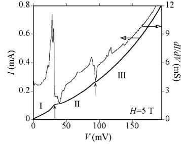
Fig. 3. IVC and  $dI/dV$  of Bi2212 single crystal mesa for  $H = 5$  T. Two kinks divide the IVC into three regions.
