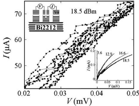
Fig. 1. Sub-branch splitting of Bi2212 single crystal mesa for  $P = 18.5$  dBm. Upper inset: schematic measurement configuration. Lower inset: IVC for various microwave-irradiation power, figures denote the power level in dBm.
