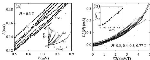
Fig. 2. (a) Sub-branch splitting of Bi2212 single crystal mesa for  $H = 0.3$  T. Inset: IVC for various  $H$  values. (b) Rescaled IVC for  $H = 0.3$ – $0.77$  T. Inset:  $V_0$  vs  $H$ .
