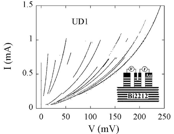
Fig. 1. Zero-field  $I$ - $V$  curves taken at  $T = 4.2$  K of the mesa UD1 which contains 12 intrinsic junctions. Inset: a four-terminal measurement configuration for the central mesa of the lateral dimensions of  $10 \times 45 \mu\text{m}^2$ .
