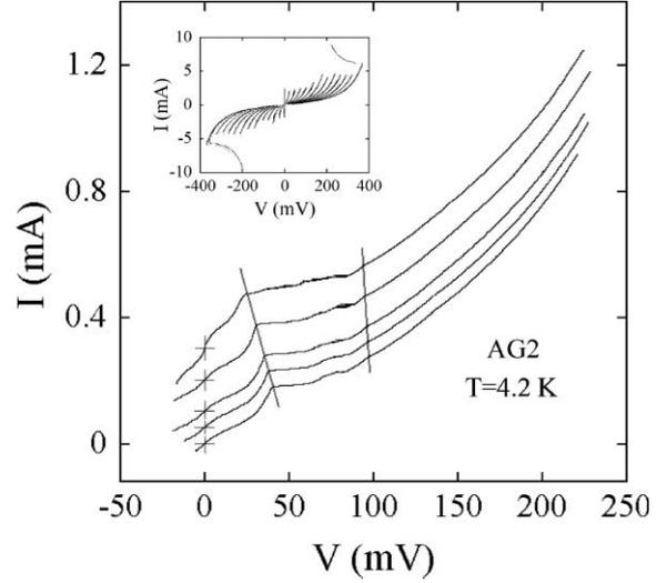
Fig. 5.  $I$ - $V$  characteristics of the mesa AG2 in dc magnetic fields of  $H = 4.0, 4.5, 5.0, 5.25,$  and  $5.5 \text{ T}$  from top to bottom. The curves for  $5.0$  and  $5.25 \text{ T}$  ( $4.0$  and  $4.5 \text{ T}$ ) are shifted upward by  $0.05 \text{ mA}$  ( $0.1 \text{ mA}$ ) from the adjacent curves for the clarity of illustration. Inset:  $I$ - $V$  characteristics of AG2 in zero external field.
