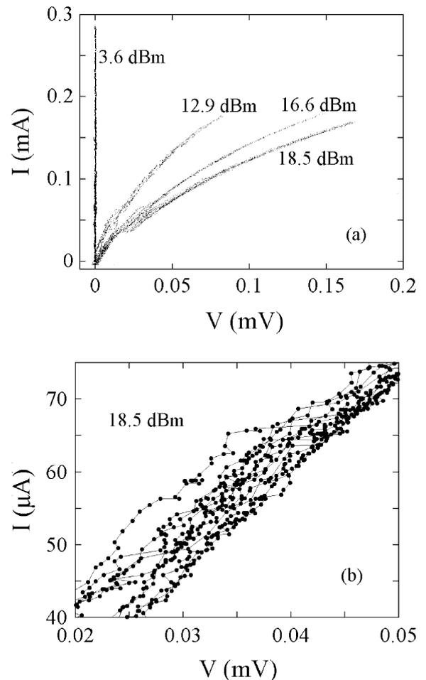
Fig. 2. (a) The evolution of the ‘supercurrent’ branch of the mesa UD1 at  $T = 4.2$  K with increasing the irradiation power of a 76 GHz microwave. (b) An enlarged view of the multiple sub-branches for  $P = 18.5$  dBm. The lines are guides to the eyes.
