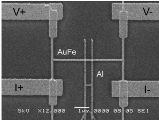
**Fig. 1** Scanning electron micrograph of the AuFe/Al hybrid loop. An Al wire of “H” shape is in contact with a AuFe wire, making a hybrid loop at center. The length of the AuFe wire is  $4.7 \mu\text{m}$ , and the dimension of the loop is  $0.5 \times 1.6 \mu\text{m}^2$ .
