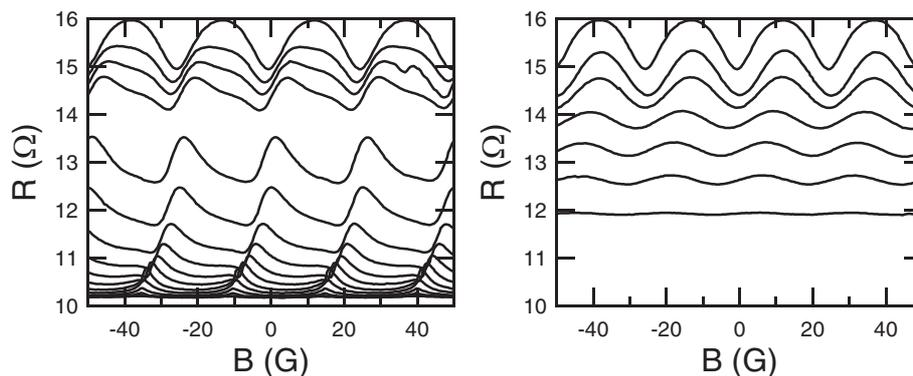
**Fig. 2** Magnetoresistance of the 26-ppm-AuFe/Al loop at various positive bias currents,  $I_{\text{dc}} = 0, 2, 4, 6, 8, 10, 12.5, 15, 17.5, 20, 22.5, 24, 25, 25.25, 25.5, 26 \mu\text{A}$  from bottom to top. The right figure shows magnetoresistance of the AuFe/Al loop at  $I_{\text{dc}} = 26, 27.5, 28, 29, 30, 31, 33 \mu\text{A}$  from top to bottom. The measurements were performed at  $T = 98 \text{ mK}$ .
