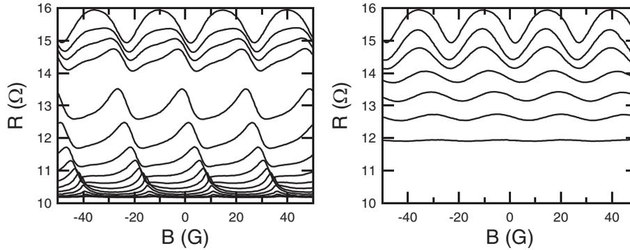
**Fig. 3** Left figure shows magnetoresistance of the 26-ppm-AuFe/Al loop at various negative bias currents,  $I_{dc} = 0, -2, -4, -6, -8, -10, -12.5, -15, -17.5, -20, -22.5, -24, -25, -25.25, -25.5, -26 \mu\text{A}$  from bottom to top. The right figure shows magnetoresistance of the AuFe/Al loop at  $I_{dc} = -26, -27.5, -28, -29, -30, -31, -33 \mu\text{A}$  from top to bottom. The measurements were performed at  $T = 98 \text{ mK}$ .
